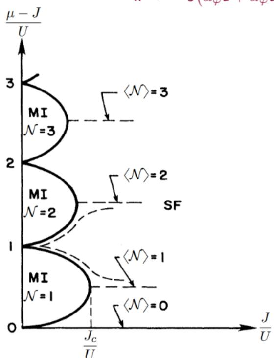
Mott insulator \ Superfluid phase diagram obtained by minimizing  $\varphi \mapsto \langle \varphi | h^\varphi \varphi \rangle$  [3]
